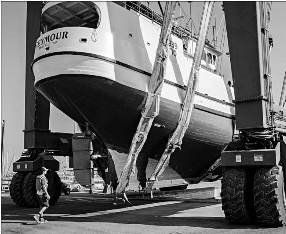
Port Townsend Boat Yard - The fishing vessel, Seymour, a halibut schooner built in 1913, is moved to the heavy haul out pier for launching. This year's haul-out included replacing three planks and re-corking 13 deck strakes along with the regular corking schedule of of four seams a year.
