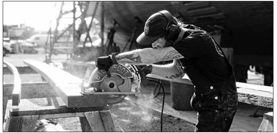
Port Townsend Shipwrights Coop - Moses Dane cuts a cover board for the well deck of the fishing vessel Vansee, a Halibut Schooner built in 1913 that is now being maintained by the Shipwrights Coop.
