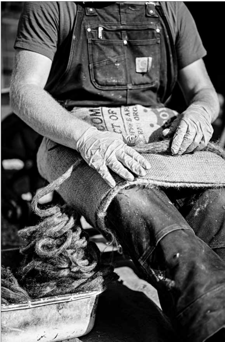
Port Townsend Shipwrights Coop - With gloved hands, Brad Seamans rolls the oil-soaked hemp oakum that will be wedged into the gaps or seams in between the planks of the fishing vessel Vansee. The oil is a combination of rape seed, flax seed, and pine tar.
