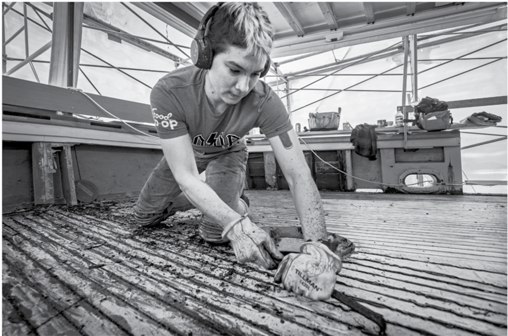
Shipwright Lou Geraghty scrapes pitch caulking from the aft deck of "Sea Wolf." Photo by Keith Thompson
