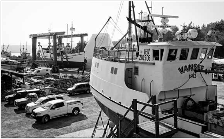
Port Townsend Shipwrights Coop - The fishing vessel Seymour is moved from the Shipwrights Coop using the 300-ton travelift to the haul-out pier for launch.
